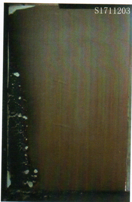
Long wing of sample, after SBI test
